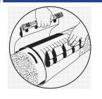
Center the EZ-MAX over the leak or damaged section of pipe till it covers the marks (step 3). Fully rotate the clamp around the pipe by pulling the nut side compression beam over, underneath, and back around the pipe.
