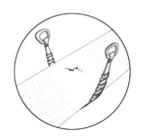
Prepare both pipe ends of the existing pipe by descaling if required. Clean the pipe as required using water. Make sure that the pipes are clear from debris and defects that may interfere with the HYMAX Outlet's proper seal.
