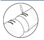
Mark the pipe ends according to the following stab depths, with two lines on each pipe end (minimum and maximum):
