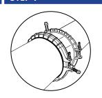
Positioning the Coupling for installation. If possible, place the coupling(s) on the replacement pipe (on both ends) and lower the pipe and couplings into the ditch. Slide the couplings outward so that they cover the minimum marks made in Step (4). Make sure there is sufficient space between the pipe ends inside the coupling so the centering pins do not touch the pipe and continuous dynamic deflection (CDD) can take place.
