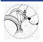
Tighten the end rings. Tighten the coupling bolts to the right torque shown on the product's label. When you finish, re-check the torque again.
