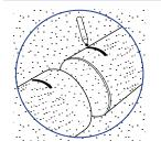
Mark each pipe end to a minimum required stab depth as indicated on the product label. This mark indicates the required stab depth for the coupling.
