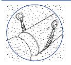
Prepare both pipe ends of the existing pipe by descaling if required. Clean the pipe as required using water. Make sure that the pipe is clear from debris and defects that may interfere with the HYMAX's proper seal.
