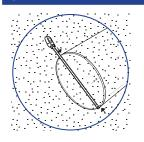
Measure the pipe's outer diameter and make sure the coupling's size will fit the pipe properly.
