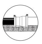
Carefully remove the HYMAX Reducer from its packaging. Inspect the coupling and end rings for shipping damage and assure that there are no missing parts.
