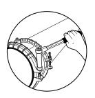
Tightening the end rings. Tighten the Reducer's bolts using a 15/16" socket wrench for 14"-24" couplings, and a 1.5" socket wrench for 26"-60" couplings. Tighten the bolts evenly on each end ring in an alternating pattern to the torque mentioned on the label. Cross-tightening ensures that the gasket is evenly seated. When you finish, re-check the torque again.
