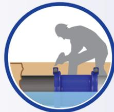
Top facing, 4-bolt and stab-on design eliminates the need for extensive under-pipe digging work, with minimum manpower, reducing time in the ditch and improving worker SAFETY.
