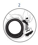
Once the ENCAPSULATION is around the pipe, engage the compression beam until it "clicks" into the 1st closing position (see below). The product can now be positioned over the leaking joint so that the 2 gasket ends are positioned on the outside of the joint on both sides according to the marks indicated in step #4.
