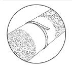
Measure the pipe TWICE using an OD tape. Select the appropriate clamp to fit the outside diameter of the pipe. Unpack it carefully.
