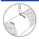
Mark the pipe according to the length of the HYMAX Tapped Clamp.
