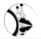
Recharge the line and check for leaks. If any leakage across the seal end is evident, reduce the pressure in the line and increase the labeled torque of the bolts up to 20%.
