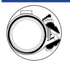
Once the HYMAX Tapped Clamp is positioned around the pipe, re-engage the side compression beam over the lug assembly by pushing it downward until it clicks in place TWICE.
