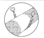
Thoroughly clean and de-scale the pipe surface where the clamp is to be installed. The pipe surface should be free of dirt, corrosion and debris.
